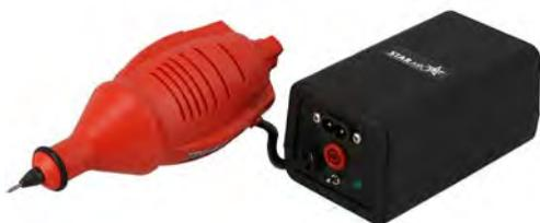
MARQUE LES MÉTAUX CONDUCTEURS PAR BRÛLAGE INDÉLÉBILE. POINTE DE 2 X 25 MM AFFUTÉE SUR LES 2 EXTRÉMITÉS. VITESSE DE MARQUAGE 6000 ÉCLAIRS/MN. LE MANDRIN S'UTILISE SANS OUTIL. ALIMENTATION PAR TRANSFORMATEUR 220/12V. ISOLATION CLASSE II. LIVRÉ EN VALISE ABS. CORPS DU GRAVEUR ABS 440 G.
